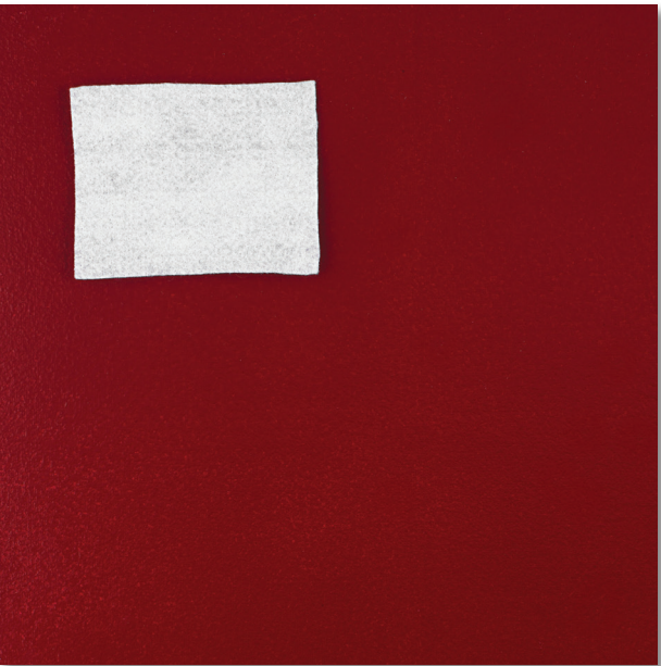
Photograph of AURA® Interior Eggshell—two coats of Caliente AF-290 over one coat of Fresh Start® High-Hiding All-Purpose Primer.
