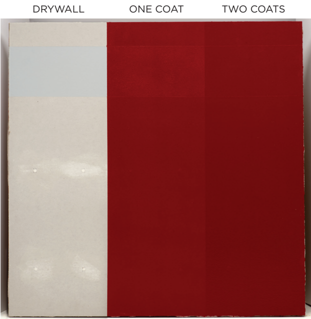
Photograph of bare sheetrock painted with one and two coats of AURA® Interior, Eggshell, Caliente AF-290.
